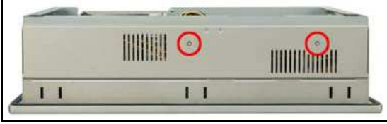
Figure 4-4: Elevated Platform Retention Screws (Right Panel)
