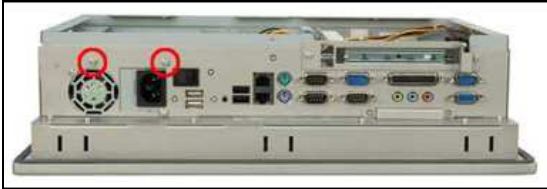
Figure 4-5: Elevated Platform Retention Screws (Bottom Panel)
