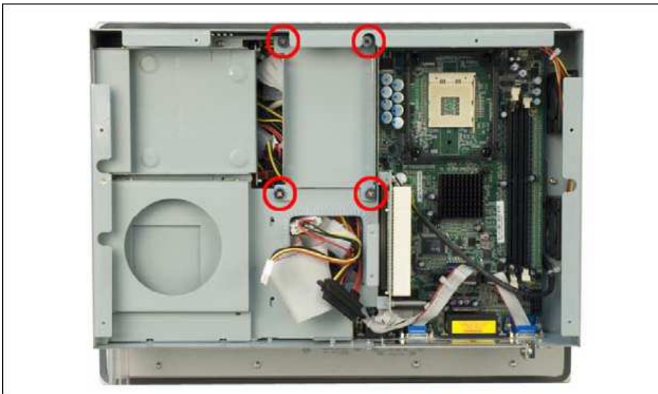
Figure 3-2: HDD Retention Screws
