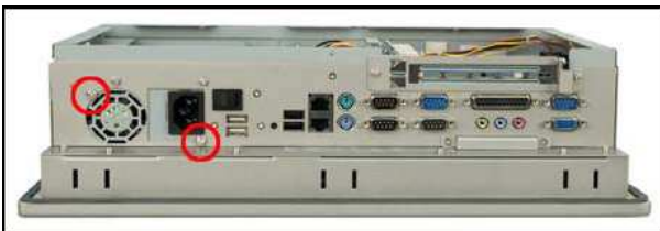
Figure 4-10: PSU External Retention Screws
