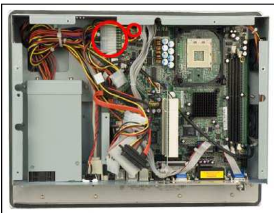
Figure 4-8: PSU Motherboard Connector
