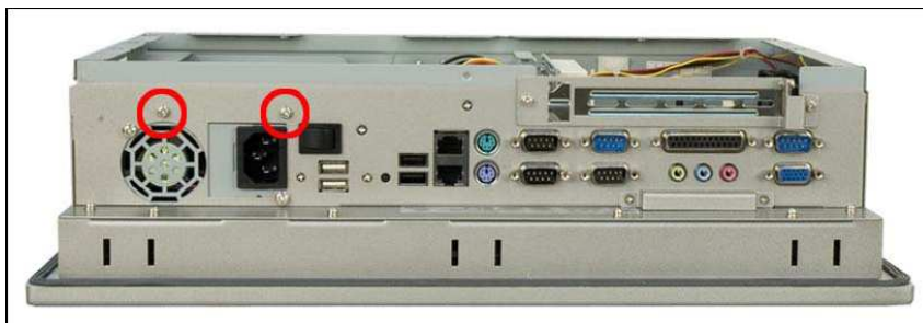
Figure 3-6: CD Drive Retention Screws
