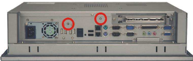
Figure 4-5: Elevated Platform Retention Screws (Bottom Panel)
