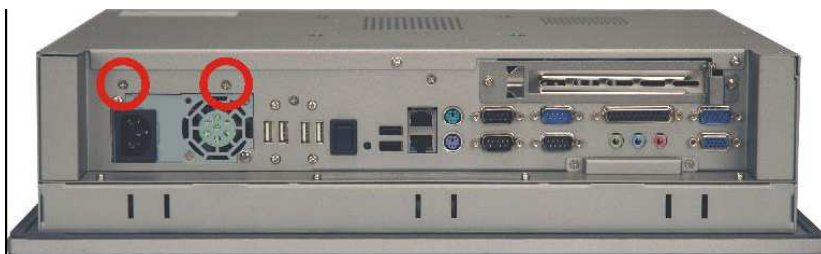
Figure 3-6: CD Drive Retention Screws
