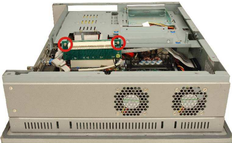
Figure 4-6: PCI Riser Card Retention Screws
